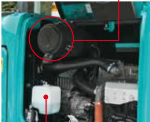
Radiator reservoir tank
