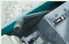
Travel high/low select switch and throttle lever
