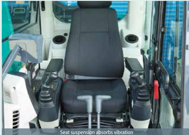
Seat suspension absorbs vibration
